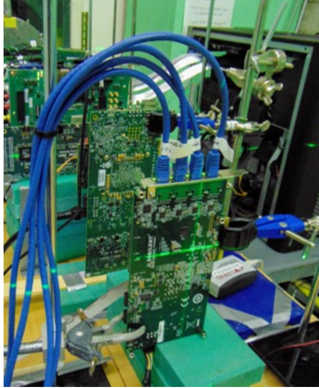
Figure 7.3: NetFPGA Positioned for Neutron Radiation Experiment
